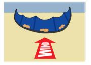
Place the kite on the ground with the top of the kite facing up, leading edge into the wind. Weigh down the canopy with some sand or a board with fins facing up.
