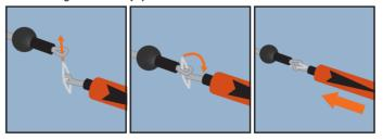
Re-connect the secondary safety release by placing the loop over the stainless steel pin, folding the pin down and sliding the relaese cuff back in place. Make sure the release cuff is sitting right against the ball after reconnecting.
